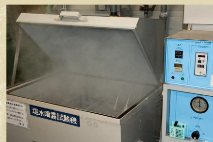
电镀硬件正在接受腐蚀性盐雾的考验
